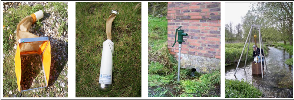
Figure 3: Methods used to collect biological samples from groundwater-dependent habitats from left: suber net, phreatic net, Bou-Rouch pump, and liquid nitrogen freeze coring.
