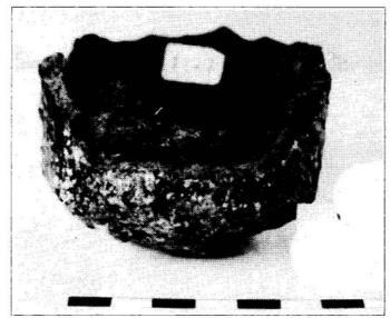
Figure 3 Lid fragment of broken wootz crucible.
