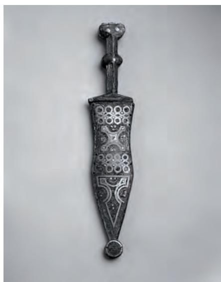
Figure 1. While the original thought is that the black patina on this dagger is niello , inspection suggests that multiple processes or steps may be responsible for the different layers of black patina 1 .
